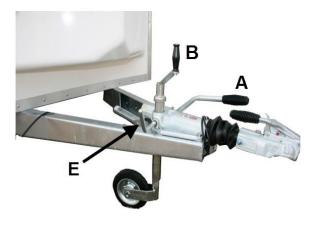
Turn the handle of the telescopic jockey wheel [B] and lower the coupling onto the ball.
