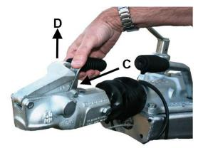
Pull back the latch **[C]** and simultaneously raise lever **[D]**, the lever will latch into position, and the coupling head can now be lowered onto the tow ball.
